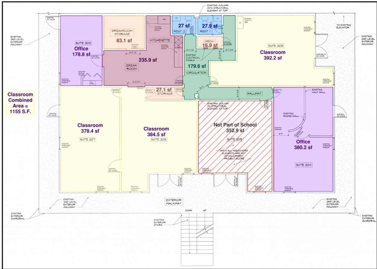
Figure 3. Suites 203, 206, & 207 Classroom Units
