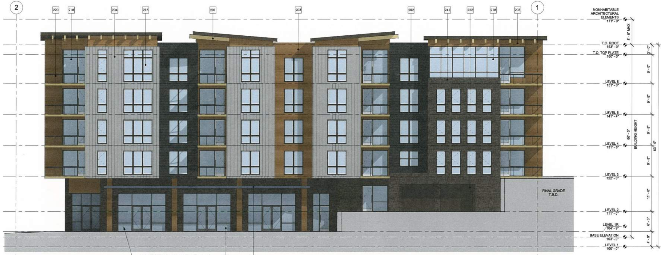
② PUD ELEVATION - EAST (LAKE DILLON DRIVE) 1/8" = 1'-0"
