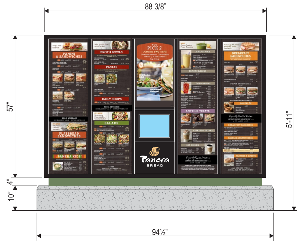
MENU BOARD ELEVATION 1/2" = 1'-0" 34.98 sq.ft. STATIC MENU COPY
