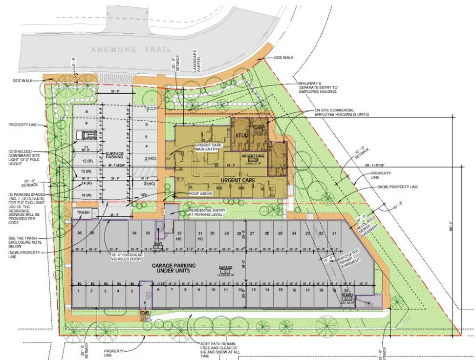
TRASH ENCLOSURE: THE STAND ALONE TRASH ENCLOSURE AS SHOWN ON SHEET A104 WILL BE PLACED IN THE CURRENT PROPOSED LOCATION AND USED FOR THE PHASE I BUILDING. DURING THE CONSTRUCTION OF THE PHASE II BUILDING, THE STAND ALONE TRASH ENCLOSURE WILL BE REMOVED AND REBUILT AS SHOWN IN THE ORIGINAL ELEVATIONS INTEGRATED INTO THE PHASE I BUILDING. BOTH PHASE I & PHASE II WILL SHARE THE SAME TRASH ENCLOSURE ONCE THE SITE IS FULLY BUILT.
