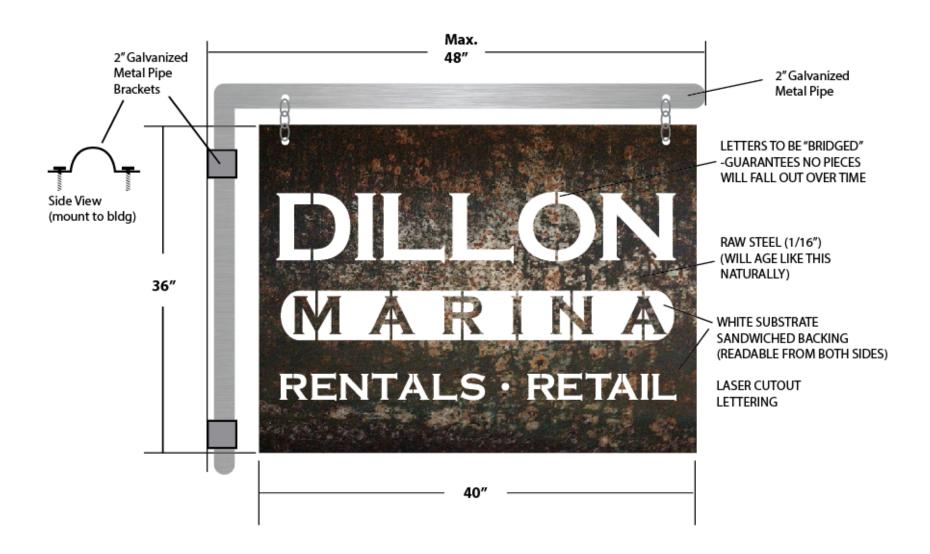
2 SIDED LASER CUT OUT LETTERING ON RAW STEEL
